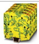
Ground modular terminal block, nom. voltage: 1000 V AC / 1500 V DC, connection method: Power-Turn connection, number of connections: 2, number of positions: 1, cross section: 25 mm² - 95 mm², AWG: 4 - 4/0, width: 25 mm, color: green-yellow, mounting type: 2.3 mm copper DIN rail
