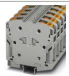
High-current terminal block, nom. voltage: 1000 V AC / 1500 V DC, nominal current: 232 A, connection method: Power-Turn connection, number of connections: 2, number of positions: 1, cross section: 25 mm² - 95 mm², AWG: 4 - 4/0, width: 25 mm, color: gray, mounting type: NS 35/15
