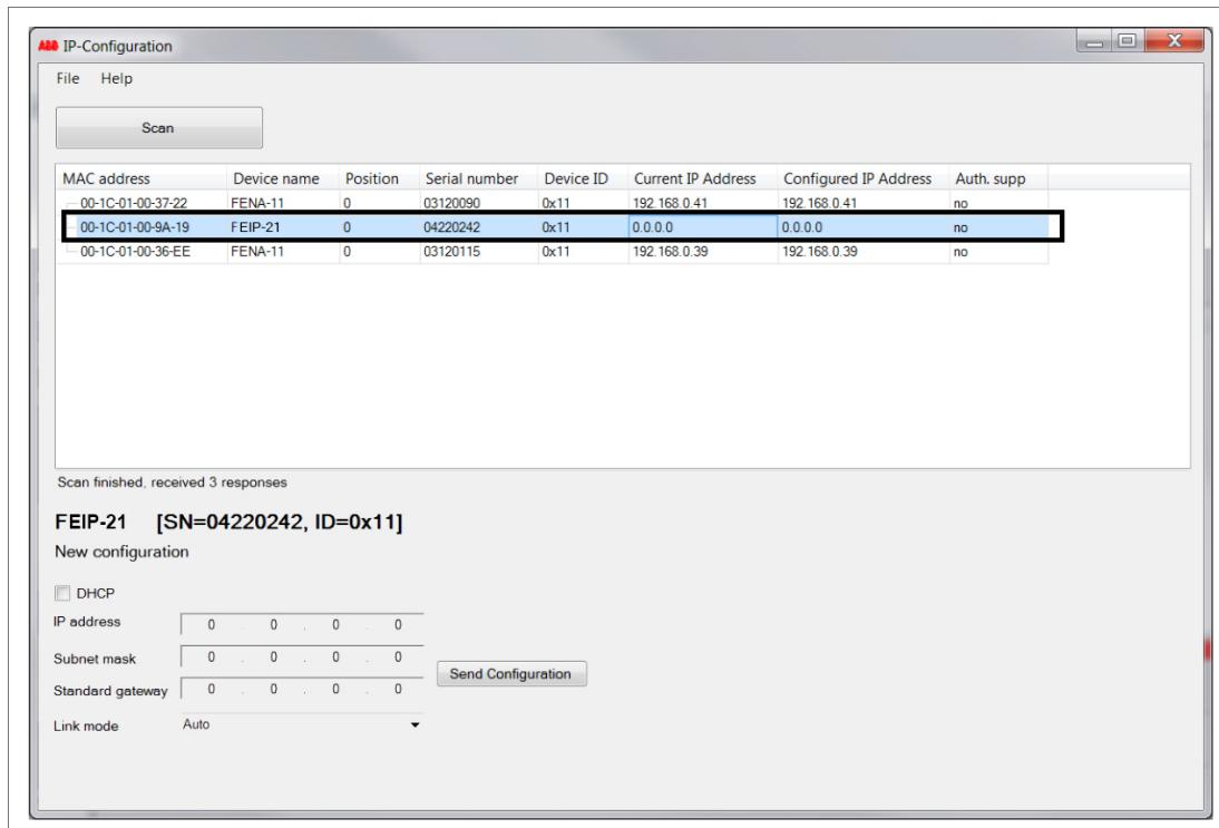
3. Below **New configuration**, define the IP configuration settings according to your network configuration.
