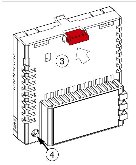
4. Tighten the screw to torque 0.8 N·m using a Torx TX10 screwdriver.
