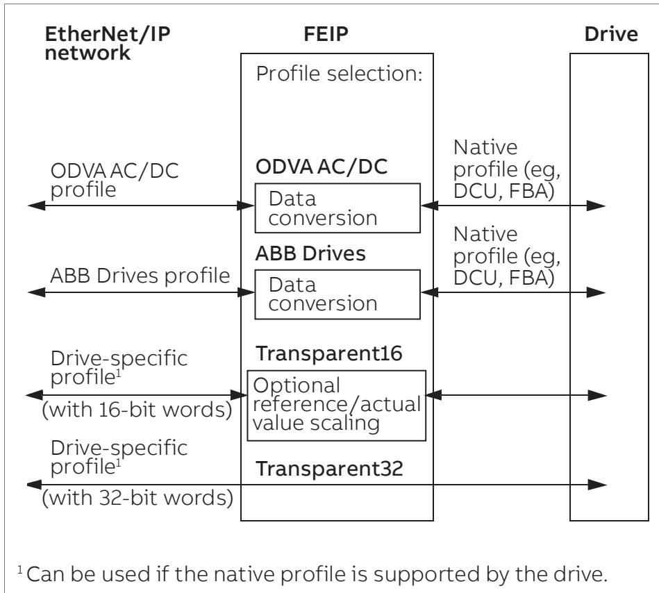
The following sections describe the Control word, the Status word, references and actual values for the ODVA AC/DC drive and ABB Drives communication profiles. Refer to the drive manuals for details on the native profiles.
