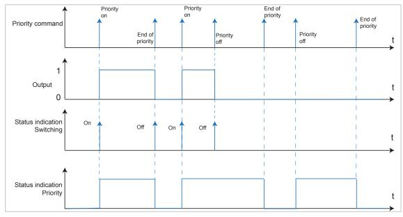
Figure 25: Signal-time diagram for Priority
