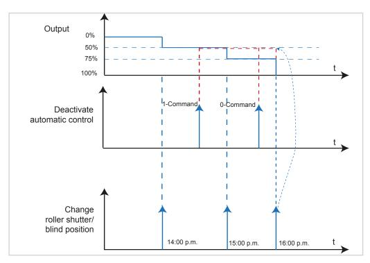
Figure 56: Signal-time diagram for Automatic control deactivation
