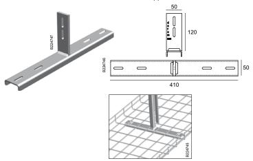
Mount the lower part of the Support Hook with 2 B2 and 2 Nut B13.
