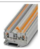
Knife disconnect terminal block, nom. voltage: 400 V, nominal current: 20 A, connection method: Push-in connection, cross section: 0.14 mm² - 4 mm², AWG: 26 - 12, length: 62 mm, width: 5.2 mm, color: gray, mounting: NS 35/7,5, NS 35/15
