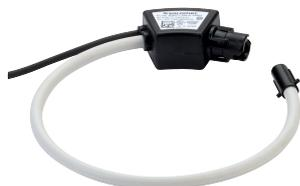
TF flexible current sensors measure the load currents of an electrical circuit and send the data to meters and Power Monitoring Devices or current modules via an RJ12 plug-and-play connection. Thanks to a wide measurement range, TF current sensors cover a wide current range from 100 to 6000 A, with only 7 references. TF flexible current sensors can be used with DIRIS Digiware I modules, DIRIS A-40 and DIRIS B.
