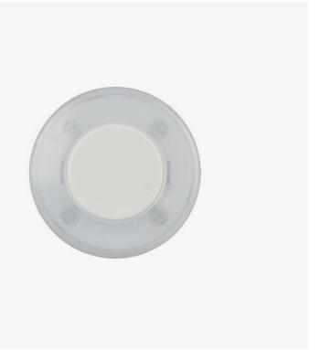
The WZ 4 status indicator is intended for optical repetition of the signalling alarming state of the detector or a group of detectors in the fire alarm systems. It can be added to the detector or a group of detectors. The indicator is applied when installed detector is invisible or there is limited access to a room supervised by detectors, for example, it is installed in spaces above ceiling, in cable passages, technical rooms, hotel rooms, etc.
