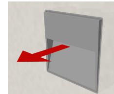
■ If needed, it is possible to remove the fixture from the backbox, simply levering under the eyelid.
