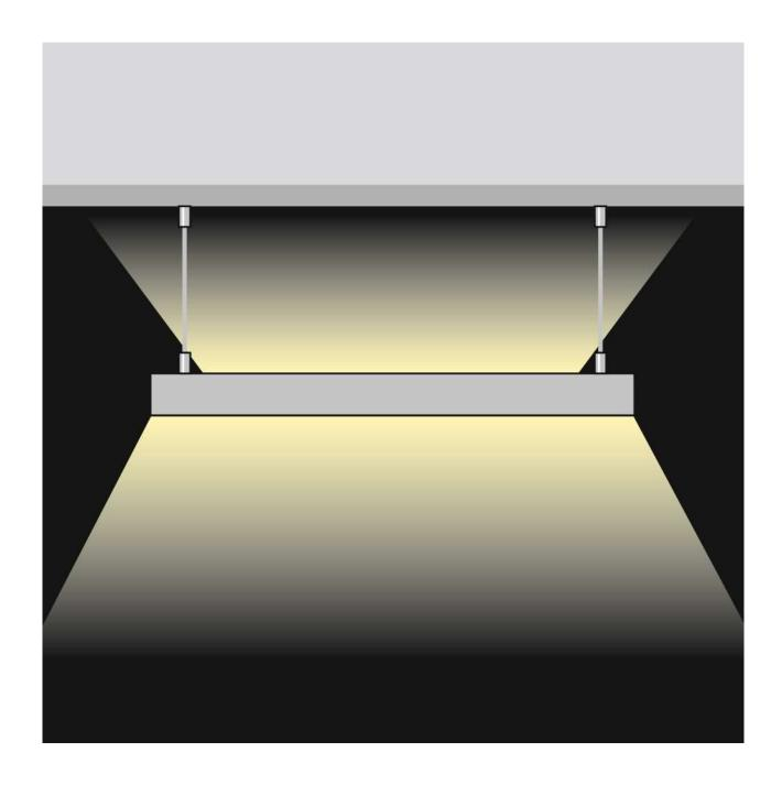
When suspended from the ceiling a doublesided installation with FLEX STRIPS is also possible (emission up- and downwards).
