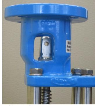
Turn spindle until the transverse spindle bore becomes visible in the recess of the adapter.
