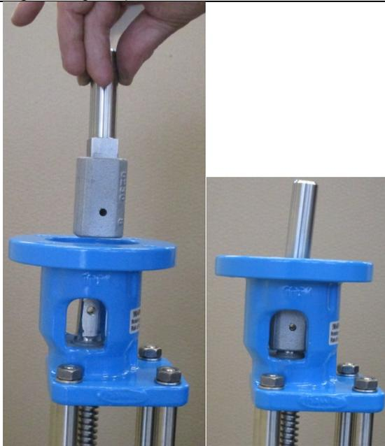
Put the spindle coupling box with the trunnion onto the spindle square in such a way that the bores coincide.
