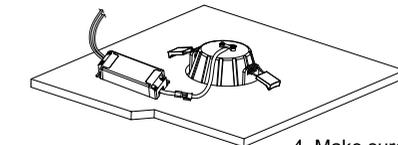
4. Make sure the downlight fixed tightly in ceiling, turn on the power (Fig 1).
