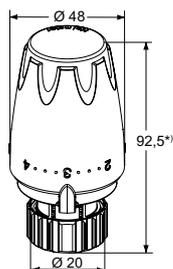
**Thermostatic head DX – For Danfoss RA**
