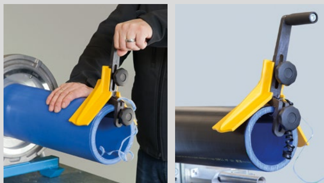
Chamfering of the front side in case of the OT and UV pipe
