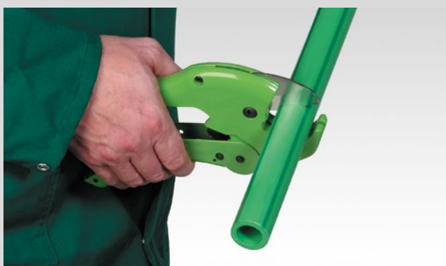
Cutting of the pipe
