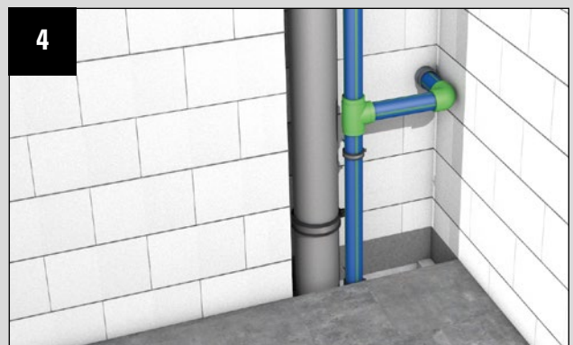
Installation of a spring leg
