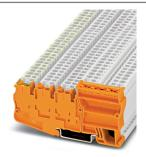
Installation ground terminal block, nom. voltage: 250 V, nominal current: 30 A, connection method: Spring-cage connection, Rated cross section: 2.5 mm², cross section: 0.08 mm² - 4 mm², mounting type: NS 35/7,5, NS 35/15, color: orange
