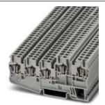
Sensor/actuator terminal block, nom. voltage: 250 V, nominal current: 18 A, connection method: Spring-cage connection, number of connections: 5, cross section:  $0.08 \text{ mm}^2$  -  $4 \text{ mm}^2$ , AWG: 28 - 12, width: 5.2 mm, color: gray, mounting type: NS 35/7.5, NS 35/15
