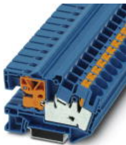
N disconnect terminal block, Push-in connection, cross section: 0.5 mm 2 - 16 mm 2 , AWG: 24 - 4, width: 10.2 mm, color: blue, mounting type: NS 35/7,5, NS 35/15
