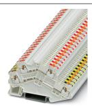
Double-level terminal block, for KNX bus in building installation, packed in pairs (25 pairs = 50 pcs.), connection method: Push-in connection, cross section: 0.14 mm² - 1.5 mm², AWG: 26 - 14, width: 7 mm, color: white, mounting type: NS 35/7,5, NS 35/15
