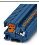
N disconnect terminal block, Push-in connection, cross section:  $0.5~\text{mm}^2$  -  $10~\text{mm}^2$ , AWG: 20 - 8, width: 8.2~mm, color: blue, mounting type: NS 35/7.5, NS 35/15
