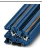
Installation terminal block, Push-in connection, cross section: 0.2 mm² - 6 mm², AWG: 24 - 10, width: 6.2 mm, color: blue, mounting type: NS 35/7,5, NS 35/15
