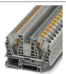
Feed-through terminal block, connection method: Push-in connection, number of connections: 2, cross section: 0.5 mm² - 25 mm², AWG: 20 - 4, width: 12.2 mm, color: gray, mounting type: NS 35/7,5, NS 35/15
