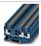
Feed-through terminal block, nom. voltage: 1000 V, nominal current: 41 A, connection method: Push-in connection, number of connections: 3, cross section: 0.5 mm² - 10 mm², AWG: 20 - 8, width: 8.2 mm, height: 42.2 mm, color: blue, mounting type: NS 35/7,5, NS 35/15
