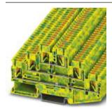
Ground modular terminal block, connection method: Push-in connection, number of connections: 6, cross section:0.14 mm² - 4 mm², AWG: 26 - 12, width: 5.2 mm, color: green-yellow, mounting type: NS 35/7,5, NS 35/15
