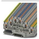
Ground modular terminal block, nom. voltage: 500 V, nominal current: 20 A, connection method: Push-in connection, number of connections: 6, cross section: 0.14 mm² - 4 mm², AWG: 26 - 12, width: 5.2 mm, color: gray, mounting type: NS 35/7,5, NS 35/15
