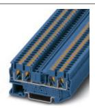
Feed-through terminal block, connection method: Push-in connection, number of connections: 4, cross section:0.14 mm² - 4 mm², AWG: 26 - 12, width: 5.2 mm, height: 35.3 mm, color: blue, mounting type: NS 35/7,5, NS 35/15
