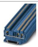
Feed-through terminal block, connection method: Push-in connection, number of connections: 3, cross section:0.14 mm² - 4 mm², AWG: 26 - 12, width: 5.2 mm, height: 35.2 mm, color: blue, mounting type: NS 35/7,5, NS 35/15
