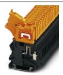
Disconnect terminal block, With test socket screws for insertion of test plugs, Connection type: Screw connection, Cross section: 0.14 mm² - 6 mm², AWG: 26 - 10, Nominal current: 20 A, Nominal voltage: 500 V, Length: 57.8 mm, Width: 6.2 mm, Color: black/orange, Assembly: NS 35/7,5, NS 35/15
