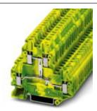
Ground modular terminal block, connection method: Screw connection, cross section: 0.14 mm² - 6 mm², AWG: 26 - 10, width: 6.2 mm, color: green-yellow, mounting type: NS 35/7,5, NS 35/15
