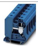
Feed-through terminal block, Connection method: Screw connection, Cross section: 1.5 mm² - 50 mm², AWG: 16 - 1/0, Width: 16 mm, Height: 65.1 mm, Color: blue, Mounting type: NS 35/7,5, NS 35/15
