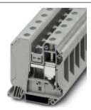
Feed-through terminal block, Connection method: Screw connection, Cross section: 1.5 mm² - 50 mm², AWG: 16 - 1/0, Width: 16 mm, Height: 65.1 mm, Color: gray, Mounting type: NS 35/7,5, NS 35/15
