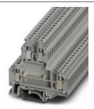
Double-level terminal block, Cross section: 0.2 mm² - 4 mm², AWG: 24 - 12, Connection type: Screw connection, Width: 6.2 mm, Color: gray, Mounting type: NS 35/7,5, NS 35/15, NS 32
