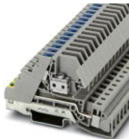
Installation ground terminal block, Screw connection, Cross section: 0.2 mm<sup>2</sup> - 10 mm<sup>2</sup>, AWG: 24 - 8, Width: 8.2 mm, Color: gray, Mounting type: NS 35/7,5, NS 35/15
