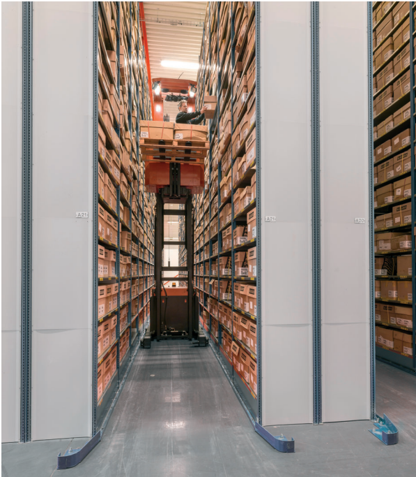
Very narrow aisle storage
