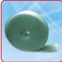
Maincor Edge Insulation is utilised around the perimeter of a room with a screeded floor to absorb expansion from the screed and prevent thermal bridging. The edge insulation also comes complete with a polyethylene section which is used to give a tight seal between edge insulation and floor insulation.
