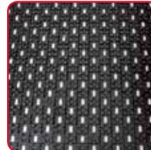
Maincor Pipe Positioning Panels are used for securing 16mm pipe within screeded floors. The castellated panels allow for the pipe to be secured at 50 - 300mm centres. Insulation is not included. The boards are to be overlapped. Each board covers an active area of (0.8m x 1.4m) 1.12m<sup>2</sup>
