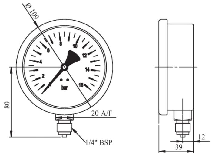
**Do not use glycerine filled gauges with any fluid which has strong oxydizing agents for example chlorine, hydrogen peroxide, nitric acid, etc.**
