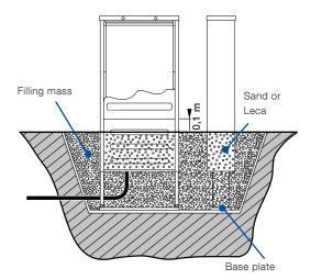
To reduce the risk of condensation we recommend filling the foundation with sand, leca and/or using a damp barrier type Cxx-DB above the foundation.
