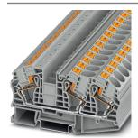
Feed-through terminal block, nom. voltage: 1000 V, nominal current: 76 A, connection method: Push-in connection, number of connections: 3, cross section: 0.5 mm² - 25 mm², AWG: 20 - 4, width: 12.2 mm, height: 53.3 mm, color: gray, mounting type: NS 35/7,5, NS 35/15
