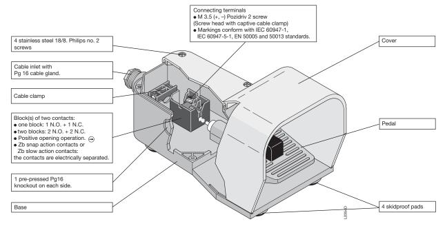
**On request:** Foot switches with covers can be assembled on a plate and equipped with a transportation handle. Instead of the handle an emergency stop button can be installed above a tube that allows for connection cable passage. (see the catalogue of separate elements)
