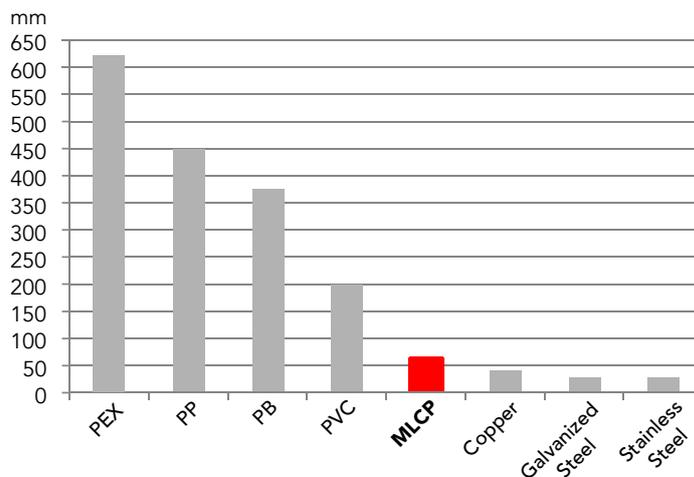
Linear expansion (mm) = coefficient of linear expansion (mm/m x K) x temperature difference (K)
