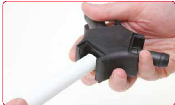
Prior to fitting connectors, the pipe is to be bevelled by inserting the beveling tool and rotating the pipe three full turns. This will put a 45° chamfer on the pipe and the pipe will be ready to take the fitting.
