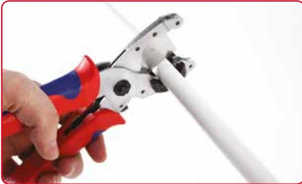
Use a set of Maincor Cutters to enable a straight and accurate 90° cut on the pipe.
