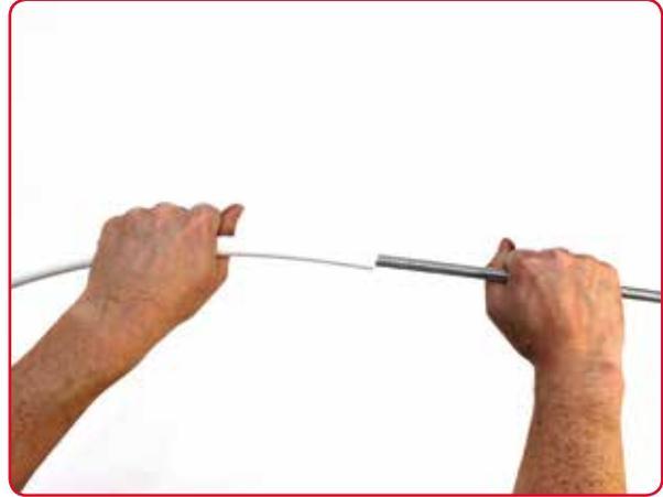
*Bending the pipe using an Internal Bending Spring.*
