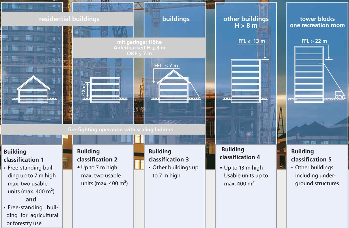
**DIN 4102 defines the requirements** in respect of the quality of walls and ceilings for fire resistance classes. The specified fire resistance class depends on the use and class of the building (see also table below).
