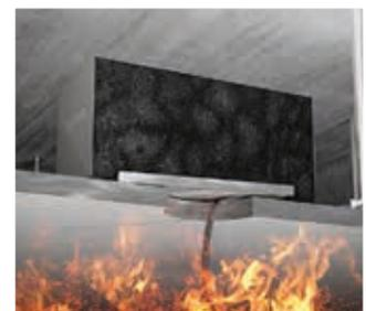
The effect of the heat causes the fire-retardant coating to tumesce, which prevents the fire and smoke from spreading.
