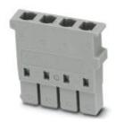
Connector housing, Connection method: Special and hybrid connection, Number of positions: 4, Cross section: 0.5 mm² - 2.5 mm², AWG: 20 - 14, Width: 5.2 mm, Height: 13 mm, Color: gray
