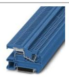
Installation terminal block, Spring-cage connection, Cross section: 0.08 mm² - 4 mm², AWG: 28 - 12, Width: 5.2 mm, Color: blue, Mounting type: NS 35/15, NS 35/7,5
