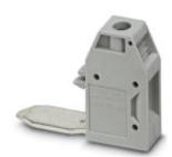
Pick-off terminal block, Can only be used in conjunction with UKH 50/70, nom. voltage: 1000 V, nominal current: 57 A, connection method: Screw connection, number of connections: 1, cross section: 0.5 mm² - 10 mm², AWG: 20 - 8, width: 10.2 mm, height: 34.7 mm, color: gray
