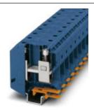
High-current terminal block, Screws with hexagonal socket, nom. voltage: 1000 V, nominal current: 232 A, connection method: Screw connection, number of connections: 2, number of positions: 1, cross section: 25 mm² - 95 mm², AWG: 4 - 3/0, width: 25 mm, height: 90 mm, color: blue, mounting type: NS 35/15, NS 32, NS 35/15-2,3
