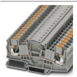
Component terminal block, for installing components that can be individually selected, connection method: Push-in connection, cross section: 0.5 mm² - 10 mm² , AWG: 20 - 10, width: 8.2 mm, color: gray
