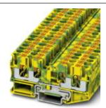
Ground modular terminal block, connection method: Push-in connection, number of connections: 4, cross section: 0.5 mm² - 10 mm², AWG: 20 - 8, width: 8.2 mm, height: 42.2 mm, color: green-yellow, mounting type: NS 35/7,5, NS 35/15
