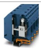
High-current terminal block, nom. voltage: 1000 V, nominal current: 309 A, connection method: Screw connection, number of connections: 2, number of positions: 1, cross section: 35 mm² - 150 mm², AWG: 2 - 300 kcmil, width: 31 mm, height: 107.3 mm, color: blue, mounting type: NS 35/15, NS 32
