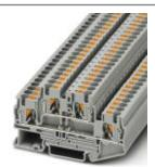
Double-level terminal block, connection method: Push-in connection, cross section: 0.2 mm² - 6 mm², AWG: 24 - 10, width: 6.2 mm, color: gray, mounting type: NS 35/7,5, NS 35/15
