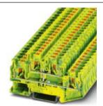
Protective conductor double-level terminal block, connection method: Push-in connection, cross section: 0.2 mm² - 6 mm², AWG: 24 - 10, width: 6.2 mm, color: green-yellow, mounting type: NS 35/7,5, NS 35/15
