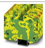
Ground modular terminal block, connection method: Power-Turn connection, number of connections: 2, cross section: 2.5 mm² - 35 mm², AWG: 12 - 2, width: 16 mm, color: green-yellow, mounting type: NS 35/15
